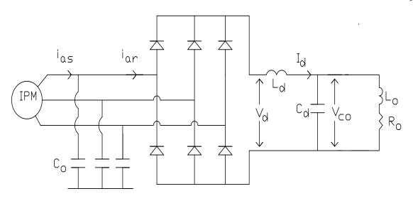
Figure 1.3. Schematic diagram of an IPM generator feediftic diagr -551.672 7 3-phase full bridge
